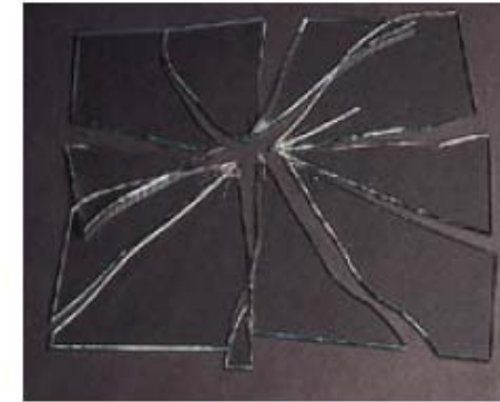
Heat strengthened breakage pattern
